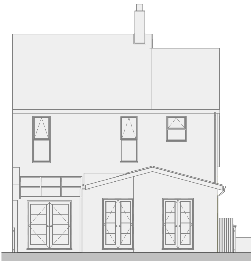
Existing Rear Elevation 1 : 100
